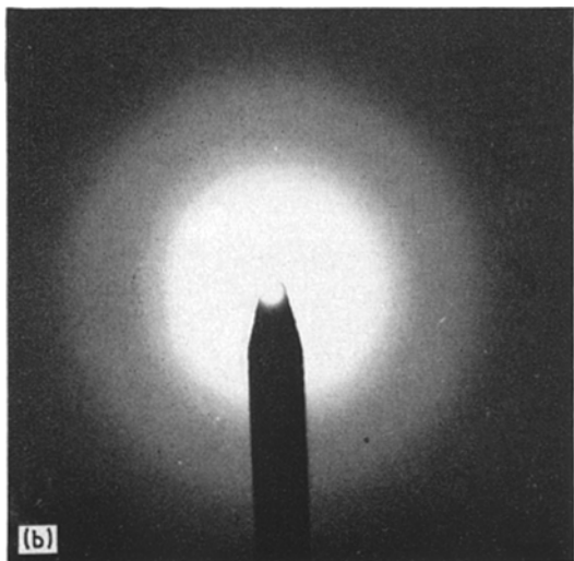
Figure 2 (a) Electron diffraction patterns from a single crystal of polyethylene at 75 kV, taken at increasing doses of irradiation. Photographic sequences such as this were used by Kobayashi and Sakaoku [80] to measure the effect of altering the beam voltage and specimen temperature. (b) Electron diffraction pattern from a single crystal of polyethylene after heavy irradiation at 80 kV (Grubb, unpublished).
